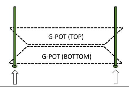
PLEASE ENSURE PART (C) IS FEED THROUGH FROM THE BOTTOM OF THE CORNER GUIDE HOLES ON THE BASE POT BEFORE ASSEMBLING.
